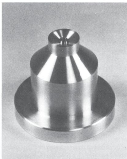
Figure 1. Standard Ford viscosity cup.
