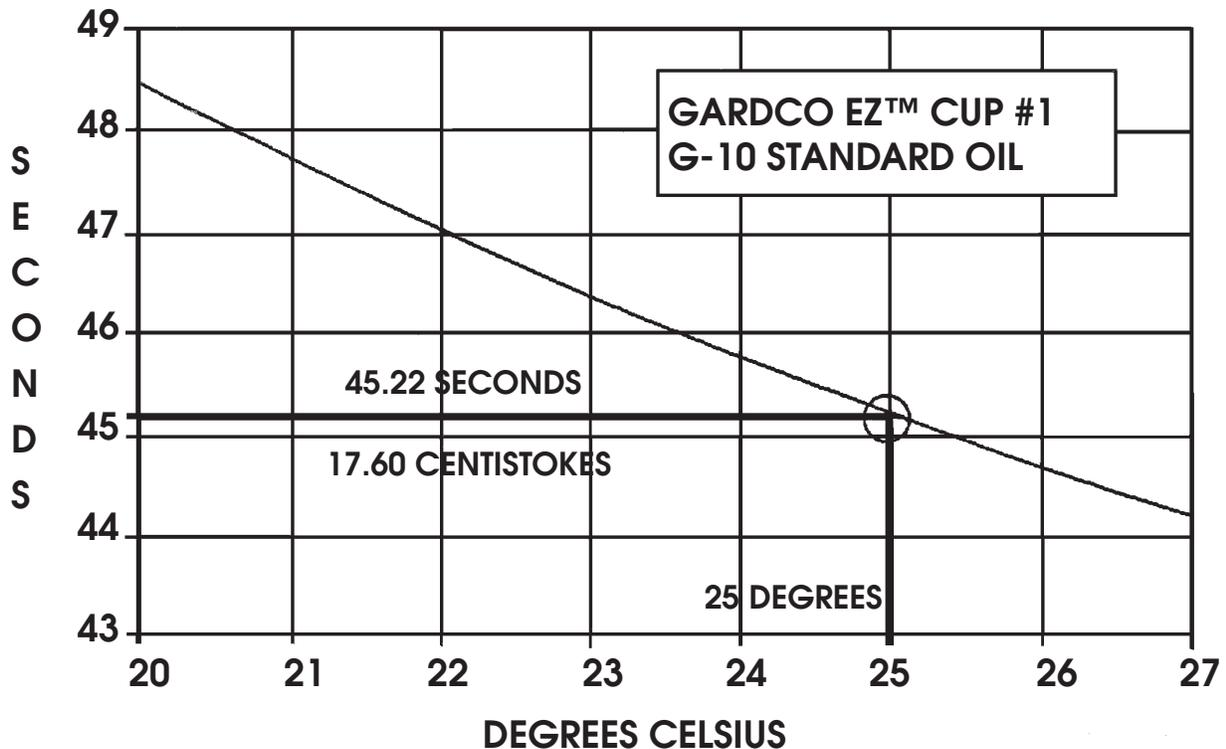
Gardco produced viscosity cups are calibrated with standard "G" Series oils. Centistoke viscosity of these oils is traceable to the National Institute of Standards and Technology. These oils are available from the Paul N. Gardner company.
